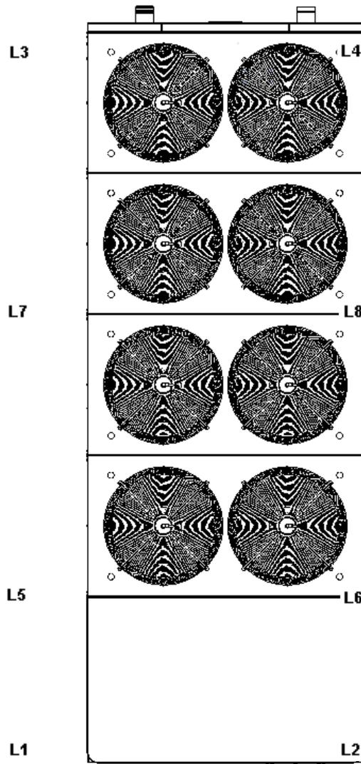
This drawing shows the points of the unit for which the **weights for the low noise version** were calculated, in configuration without pumps, without tank and empty with treated water. They are shown on the following table.
