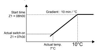
In order to ensure the unit perfectly matches the requirements of the most difficult applications in terms of occupation and varying internal loads, the new eCLIMATIC offers now up to 7 time zones per day (Z0 to Z6) adjustable by steps of 10 minutes. Each time zone can be programmed to follow one of four possible operating modes:
