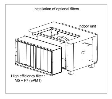
As standard, the unit are delivered with G4 filters. As an option, M5 + F7 (ePM1) filter is available.
